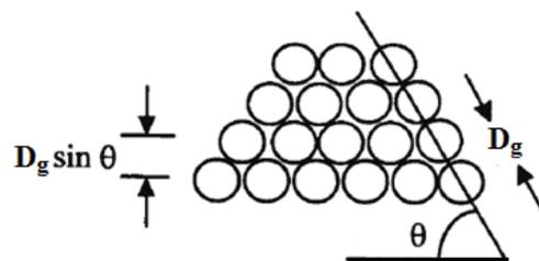
Figure 1. Rhombic stacking model for fruit
