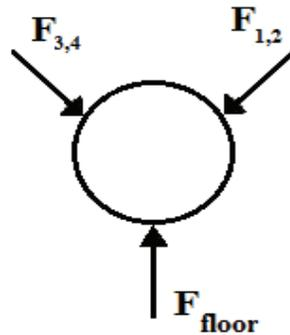
Figure 3. Static forces on the last layer of fruit
