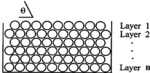
Figure 2. Diagram of stack of samples having  $n$  layers and confined by a vertical wall and a floor
