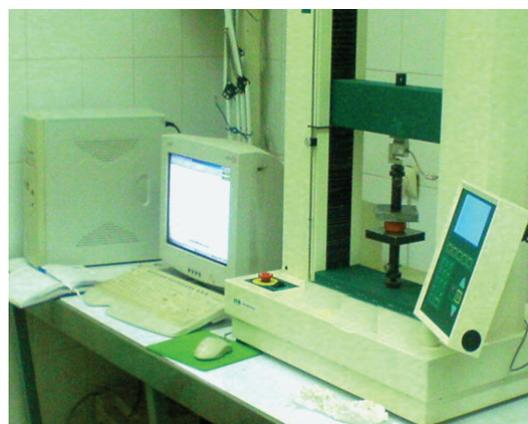
Figure 5. Universal testing machine
