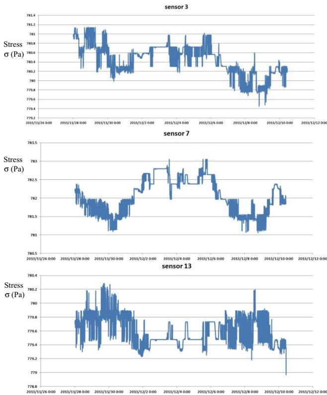
Figure 6. Stress data at selected locations on the back surface of the PV panel
