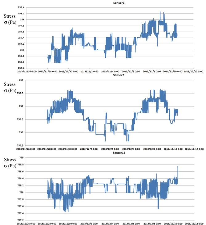
Figure 5. Stress data at selected locations on the front surface of the PV panel
