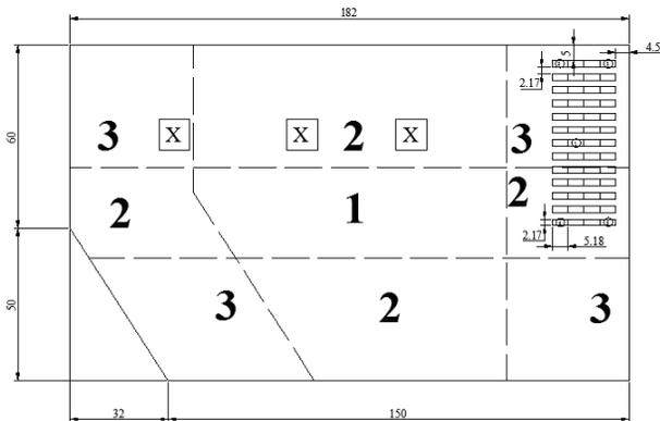
Figure 8. PV panels location on the flat-roof (SEAOC, 2013)
