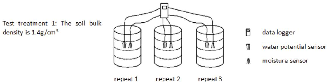
Figure 1. Design of test equipment (single treatment)
