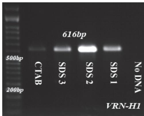
Figure 3. Agarose gel electrophoresis of PCR product obtained with HvBM5A-exon 2 primers
