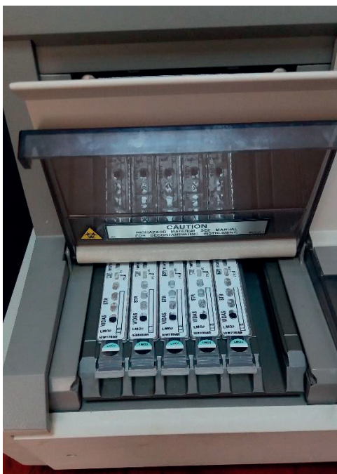
Figure 2. Performing LMO detection by using VIDAS® Listeria monocytogenes II (LMO2) (bioMérieux, Marcy-l'Etoile, France)
