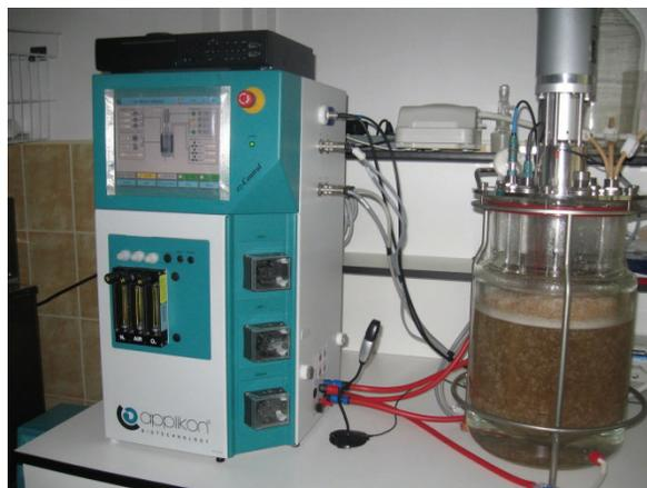
Figure 1. Laboratory-scale bioreactor for submerged cultivation of edible mushrooms
