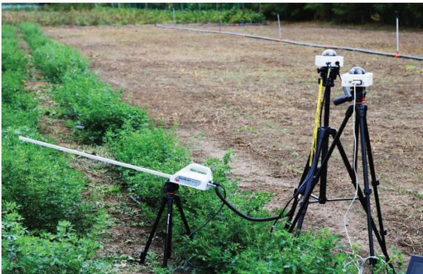
Figure 1. Monitoring of light interception and absorption in alfalfa canopy using a Delta-T Devices SunScan SSI canopy analyzer and beam fraction sensors; 27 varieties have been screened for solar radiation patterns
