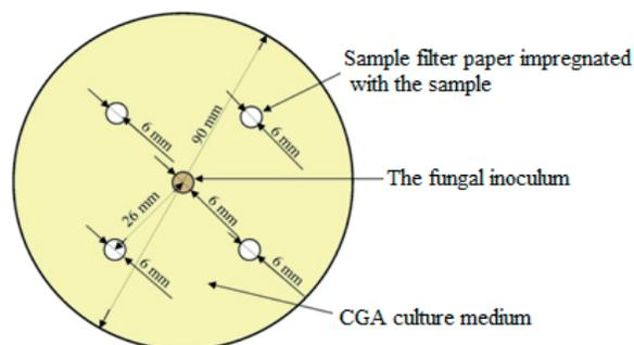
Figure 1. Essential oils inoculation model for testing antifungal activity
